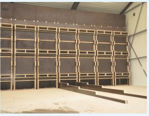
A way to dry bulbs fast and equally is by using sloping beams. The boxes are placed on descending beams in front of the air outlet of the system. This makes the air distribution consistent. The air is forced through the bottom of the box. An advantage of this system is that the boxes can easily be placed in front of the system with a fork-lift. A disadvantage is that this method needs more space (piling boxes is not possible).
